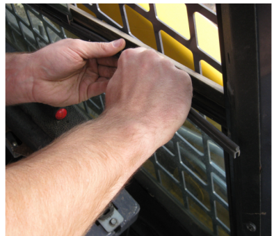
Figure 1 Rail removed from window frame.
