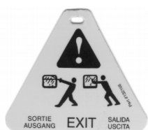
132166 – Located on rear window emergency exit
