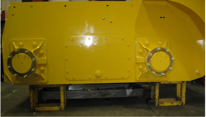
Figure 2 Loader Properly Blocked
